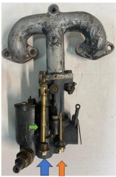
The brass jets have been placed outside the carburettor body, to illustrate their relative positions. The slow-running/compensating jet is on the left (blue arrow), together with the mixture jet (green arrow) with the normal jet on the right (orange arrow).
